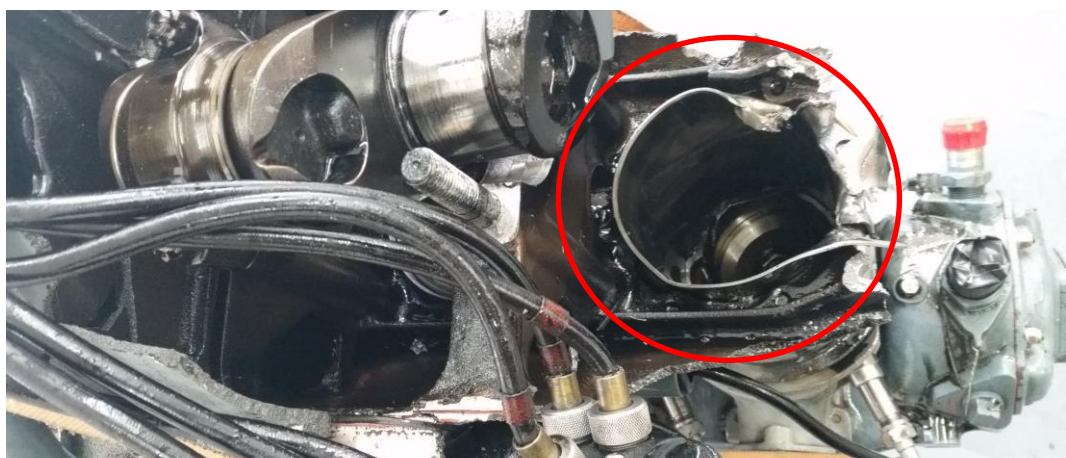
Figure 4: The components of cylinder no. 1 (marked in red), the rearmost cylinder viewed in the direction of flight, were destroyed.
